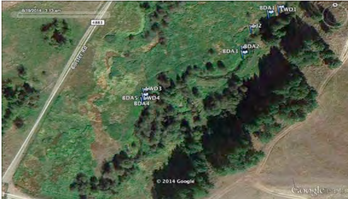
Figure 77: Myers Creek restoration site showing locations of LWD and BDA placement
